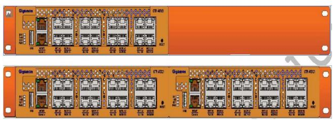
Figure 3 Rack Ears for Front Mount
